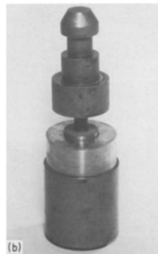
Figure 2 The special device for measuring the mechanical properties of the bonded plates: (a) schematic drawing; (b) general view.
